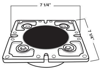
**PASCO**'s NEW Quick Set Square Closet Flange will solve the problem of properly supporting a closet flange mounted in a square hole. Keep in mind that the pipe doesn't support the flange, the sub-floor does. Simply push the QUICK SET CLOSET FLANGE flush on the DWV pipe and alternately tighten the four stainless steel screws. Secure to subfloor with brass wood screws.
