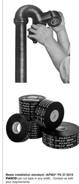
**PASCO**'s "All Weather" Pipe Protection Tape is a tough PVC plastic tape with special high tack adhesives formulated to resist corrosion. It is easy to apply by hand with no special tools or equipment. It provides positive protection against abrasion and corrosive action for steel pipe, fittings & electrical conduit systems.
